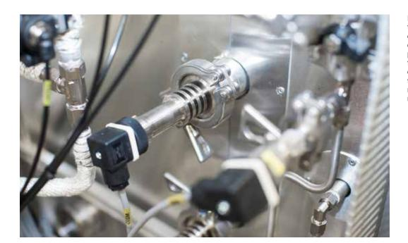
PBMH pressure sensor in the BST sterilizer system chamber. Cooling fins on the sensor isolate process temperature from the electronics, enabling use in a high temperature environment with no time restrictions.
