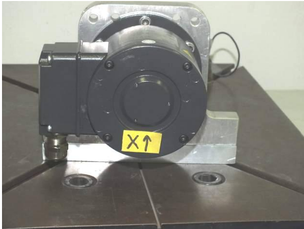
picture 7 Incremental Encoder POG 9 on the shock table with acceleration sensor during shock test in X-axis, positive direction
