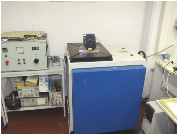
picture 9 Incremental Encoder POG 9 on the shock table with acceleration sensor during shock test in Y-axis, positive direction
