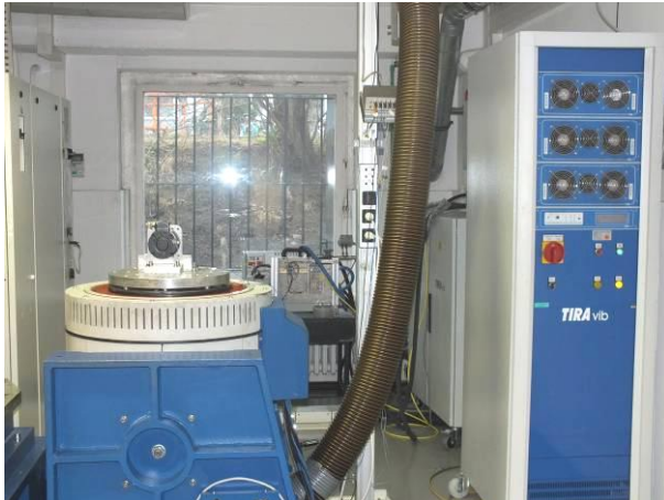
picture 3 Incremental Encoder POG 9 specimens on the vibration test device during vibration test in Y-axis
