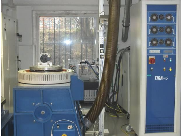
picture 1 Incremental Encoder POG 9 on the vibration test device during vibration test in X-axis
