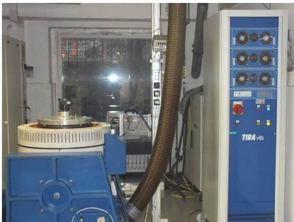
picture 5 Incremental Encoder POG 9 specimen on the vibration test device during vibration test in Z-axis
