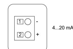
Device supply is via the 4...20 mA current loop.
