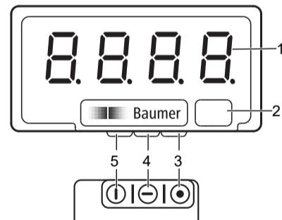
After power on the device is in **RUN** mode. The current value (actual value) is displayed.
