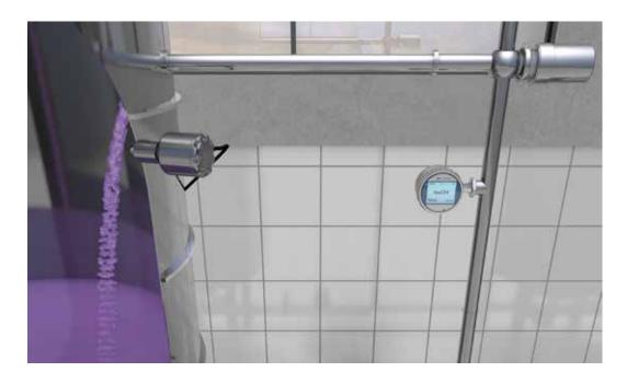
To control concentrate dosing of acid or caustic substances, the conductivity transmitter measures the specified concentration. With precise measurement it ensures food safety and savings of cleaning agent usage. Due to its robust hygienic designed tip, it survives with a long life cycle.
